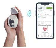
The Propeller EMM attaches to the ELLIPTA inhaler to track medication usage. Data collected by the EMM is sent wirelessly via Bluetooth to a paired smartphone app.
